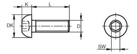
Dimensions of Metric ISO 7380-1 Button Head Hexagon Socket Cap Screw
