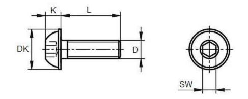
Dimensions of Metric ISO 7380-2 Button Head Hexagon Socket Cap Screw With Collar
